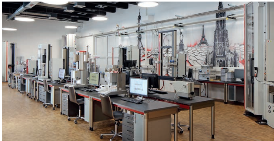
Fig. 2. Static testing machines and instruments in the ZwickRoell testing laboratory
