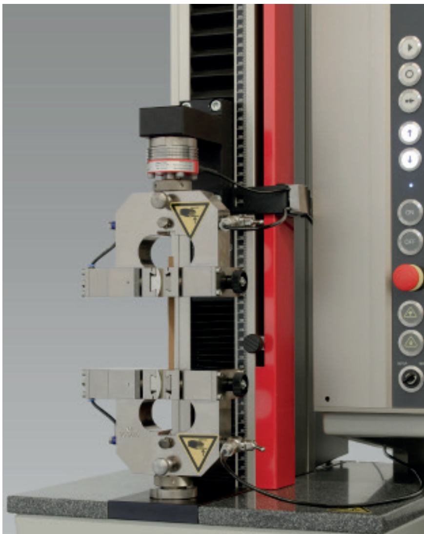
Fig. 1. Dry tensile test on paper
