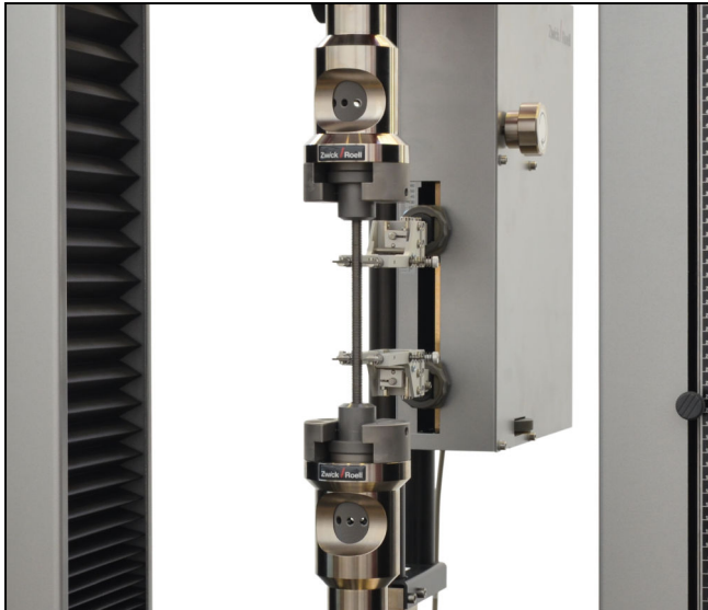
Specimen grips for dumbbell, threaded and threaded-end specimens Type 8496, Fmax 50 kN
