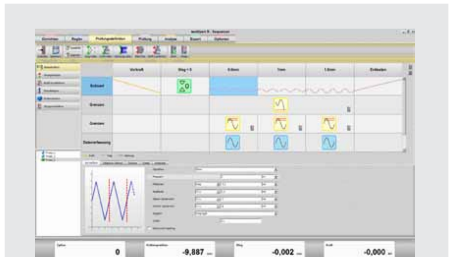
Fig. 2: Test sequence definition (block programming)
