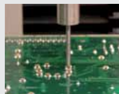
Testing of soldered pins
