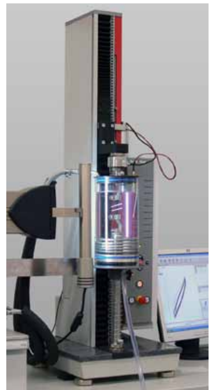
Fig. 4: Tensile test at 37 °C (+ water-bath) with video extensometer
