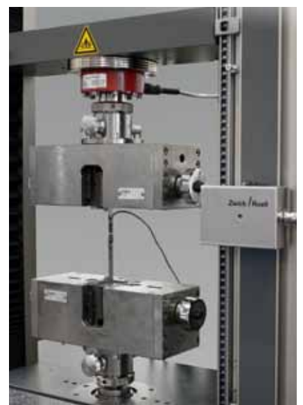
Fig. 5: Strain gage connected directly to testControl II via a pre-configured in-line switchbox
