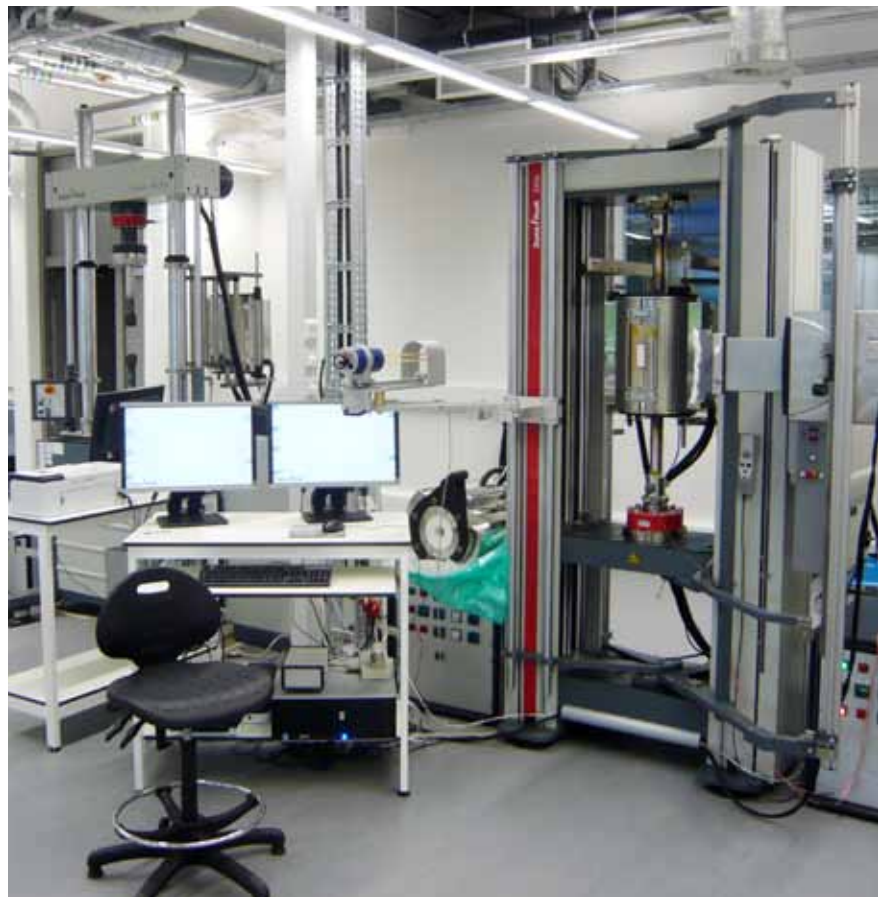
Fig 3: AFRC, Advanced Forming Research Centre, University of Strathclyde: High-temperature testing (static and dynamic)
