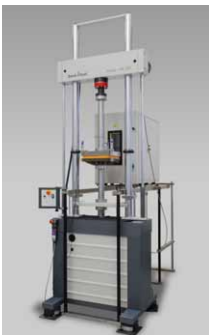
Fig. 1: Servo-hydraulic testing machine with high-temperature furnace
