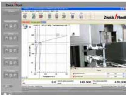
Fig 1: The video picture and the data curves are exactly synchronized
