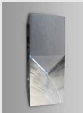
Fig. 4: Fractured specimen, display showing force, crack length, R+a/W, stress intensity, crack growth and crack growth per dK
