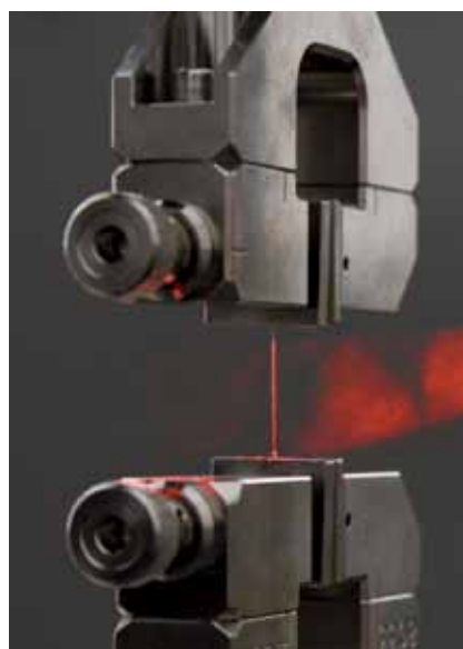
Fig. 2: Non-contact extension measurement with laserXtens, also suitable for micro-specimens
