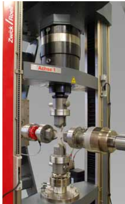
Fig. 2: Biaxial testing machine with superimposed torsion
